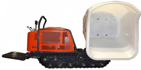
CANYCOM BUGGY 20 HP HONDA SWIVEL BUCKET 16 CU FT BUCKET
